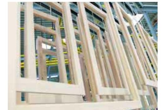
If the assembled frame is impregnated, there is no protection in the connection areas.
