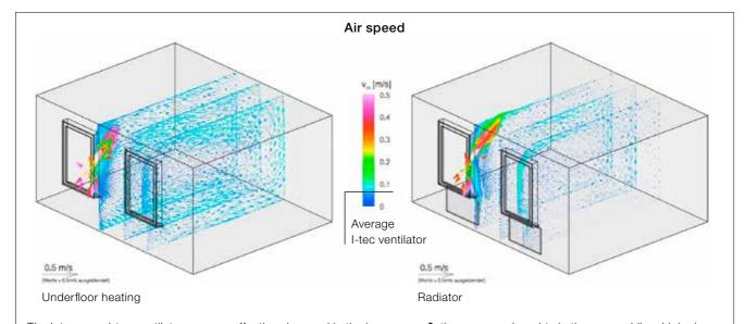
The Intermorm I-tec ventilator ensures effective air speed in the lower area → there are no draughts in the room while a high air exchange occurs (independent of underfloor heating or radiators).
